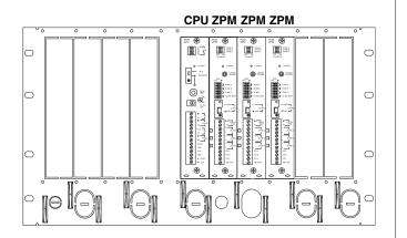
A 15-zone PCM system without talk-back capability, six-zone slave assembly mounted at left:
